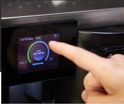
Electronic hot water button.
